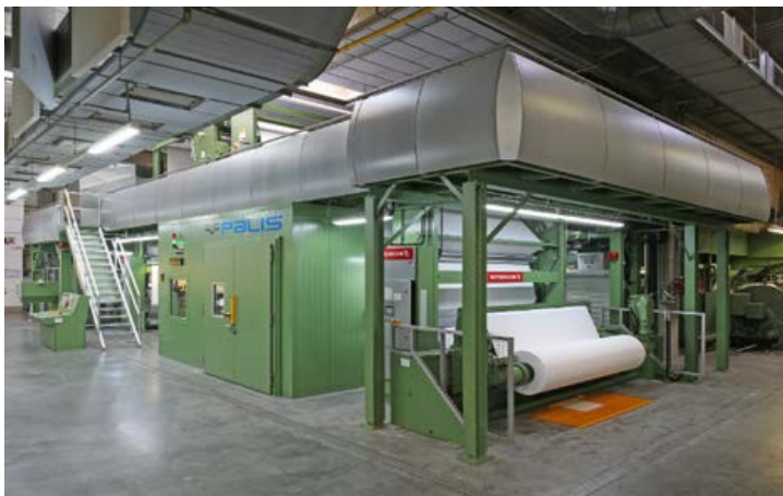
Figure: Digital printing system making Schattdecor the only company in the industry to be able to digitally print paper with a width of 2.25 meters at a speed of 163 meters per minute when it was installed in 2016.
