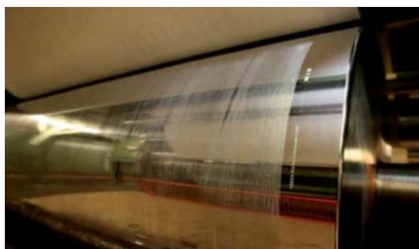
Figure: Printing cylinders with decors from Schattdecor's engraving and electroplating department
