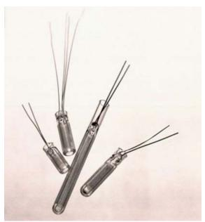
Figure 1: The patenting of the "electrical resistance thermometer made of platinum wire" by W. C. Heraeus in 1906 marks the beginning of modern temperature measuring technology. The novel design (platinum wire wound up on a piece of quartz glass and protected by a quartz glass tube) permitted the safe, accurate and fast measuring of high temperatures.
