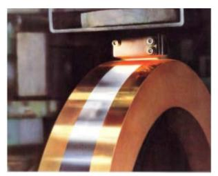
Figure 4: Melt spinning process
