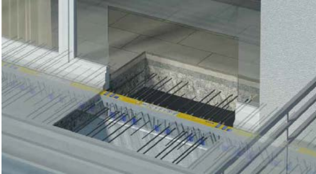
Figure 3: Cross-section of the installation situation of an Isokorb® between ceiling and balcony
