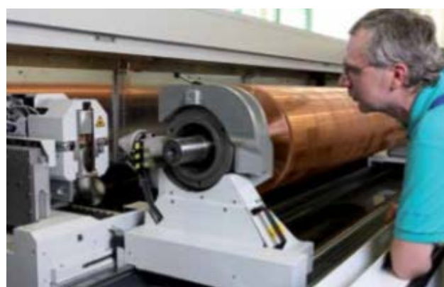
Figure: Copper-plated steel cylinders being engraved with a laser for printing
